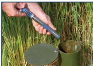
The **LevelLine-ECO** from **AQUAREAD™** is a water level and temperature recording device that has been specifically designed for long term water level logging. Designed to be deployed and left unattended in the field for long periods of time, the stainless steel LevelLine-ECO is the cost effective way to get into water level logging.
